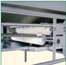
Rotary brushes and a hot water rinse continuously clean the conveyor belt.
